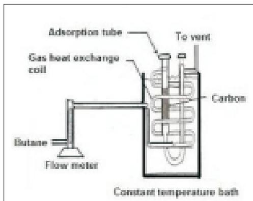
Picture 4: **Apparatus for Butane activity test**
