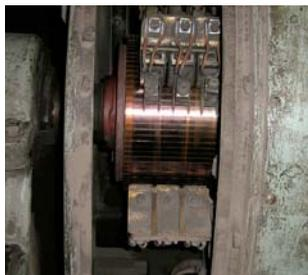
Metallic and chemical contaminants along with abrasive dust and dirt will attack the electrical insulation qualities of the motor/
