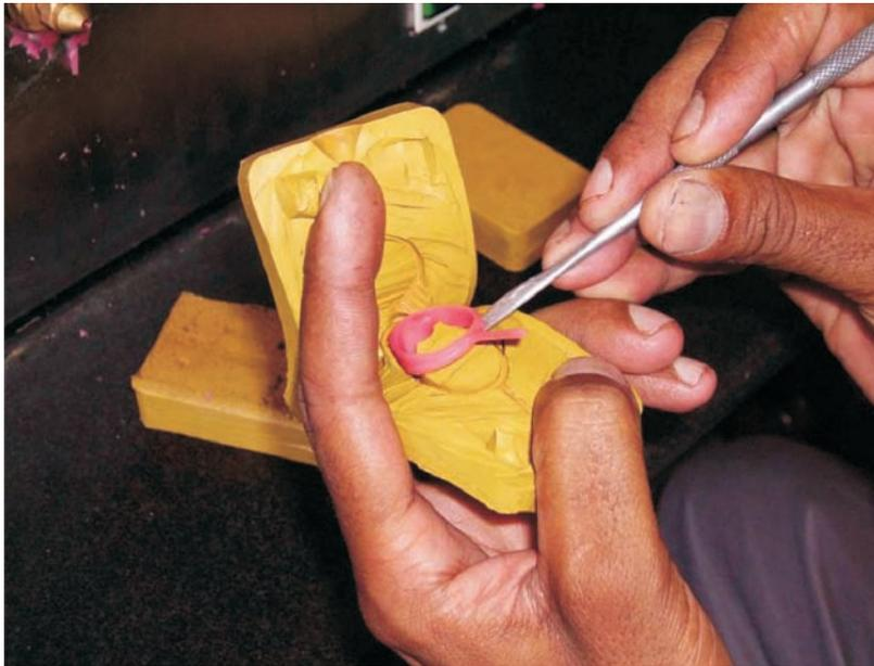
Picture 1: Making the Mould
