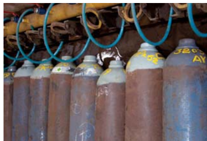
Picture 5: Cleaning of cylinders with aqueous solution and drying with warm nitrogen
